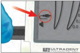
1. Plug the measuring cable into the device. The connector icon will appear.
